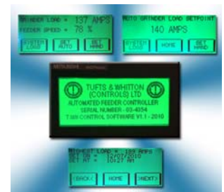
Grinder Feeder Touch Screen Control
